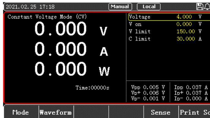
Figure 4-1-2-1 Setting Interface of CV Mode
